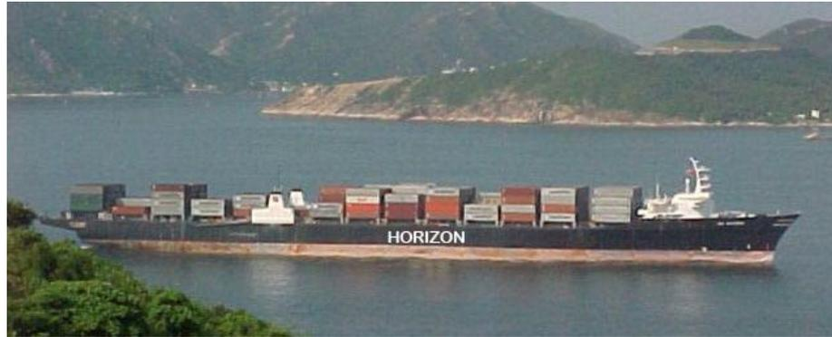
The *Spirit* is 272 m long and 30 m wide, with a maximum speed of ~20 knots.
